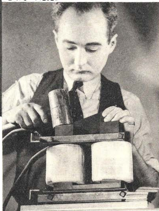
The remaining pieces of iron are woven into the open end of the core and then bolted between the two angle-iron supporting pieces, as shown above.
