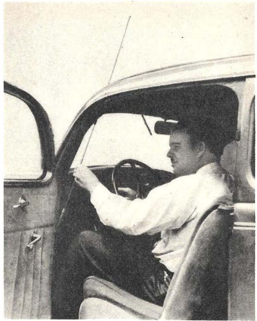
No longer is it necessary to get out of the car to adjust the "buggy whip" antenna. This new type can be raised or lowered quickly and easily from the inside.
