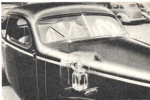
Above — Smeared or dirty windshields will be a thing of the past when this automatic windshield washer is used.
