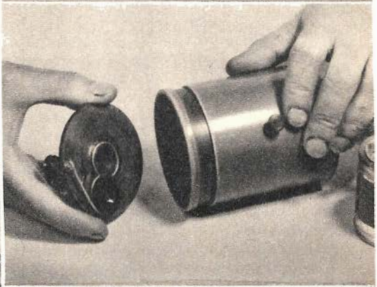
Left—Parts for the lamp-house, and the toy train transformer used for power. Above—How the Bakelite lens disc is cemented into the focusing tube. Notice the simple red filter, which covers the lens while the enlarging paper is being positioned.
