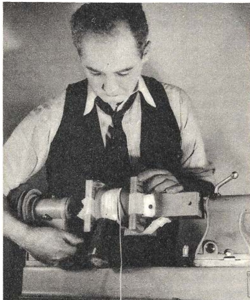
Left—Tap each layer of wire neatly in place with a rubber or wood mallet. Right—By tapping the end of the tapered wood core on a hard surface, coil will slide off easily. Ends of gauze strips are tied to hold windings intact.
