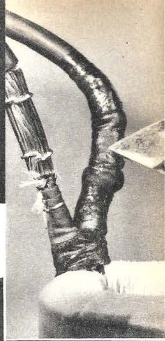
Left—Covering the coil with cotton gauze. The outside of each coil then is coated with white shellac. Right—The three wires from each end of the secondary are soldered to the heavy electrode and ground cables.
