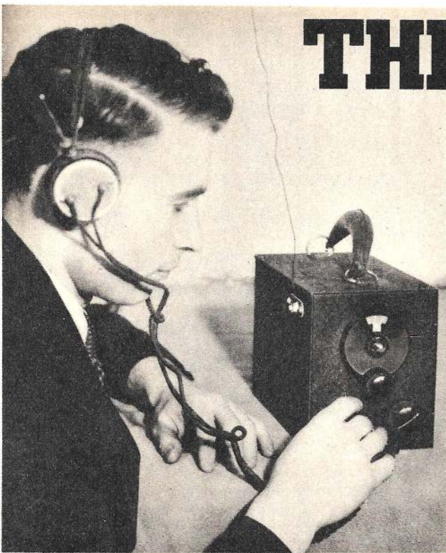
The completed set in use. The binding post at the left is for the antenna connection. All batteries are in the cabinet.
