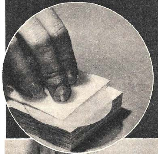
Top—Riveting the hinges to the Bakelite negative holders. Above—Cementing the glass sheets in place. Old glass plate negatives are suitable for the purpose.
