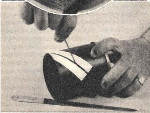
Circle—Grinding the round diffusion glass with valve grinding compound and water. Left—The slot in the inner focusing tube is cut with a short piece of scroll saw blade, and smoothed with the nailfile.
